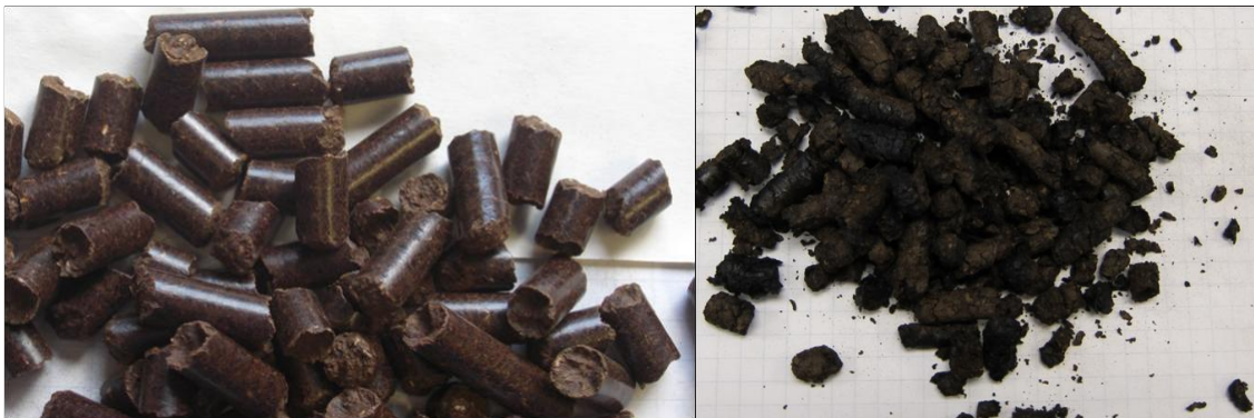
Figure 4-2 Steam explosion pellets (l) and torrefied pellets (r) after weathering
