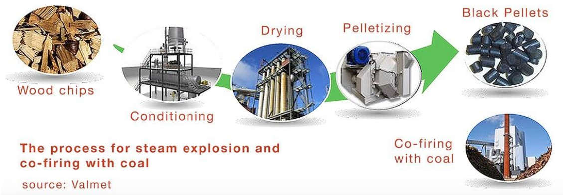
Figure 2-2 simplified steam explosion process by Zilkha.
